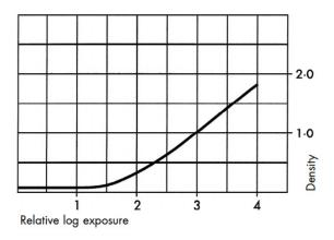
100 DELTA Professional roll film developed in ILFORD ID-11 stock for  $8\frac{1}{2}$  minutes at  $20^{\circ}\text{C}/68^{\circ}\text{F}$  with intermittent agitation. This curve is also representative of the 35mm and sheet film formats.
